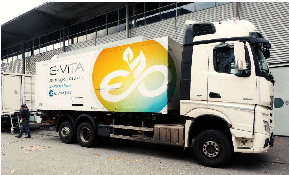
E-VITA® plant technology for efficient on-site seed treatment © E-VITA GmbH
